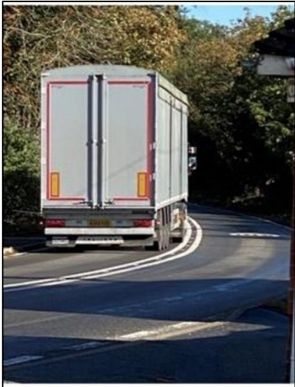
Plates 4 and 5: Standard width and length HGVs sit just within double white line system at Little Glemham
